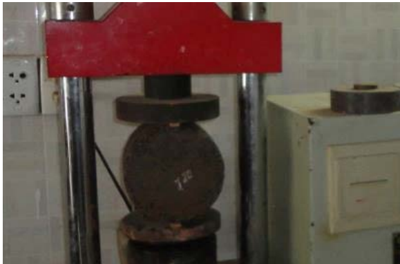
Figure 6. Splitting tensile strength.
