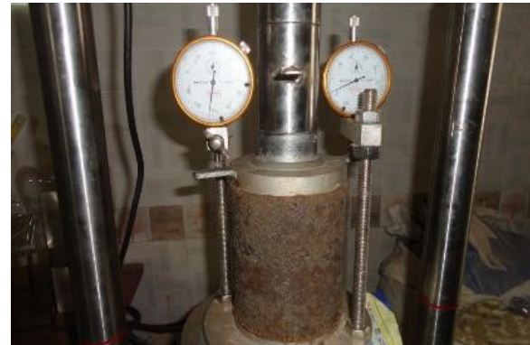
Figure 7. Elastic modulus test.
