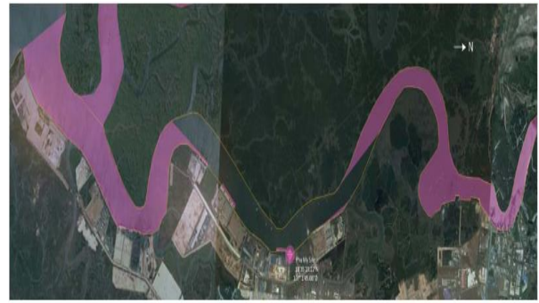
Figure 4. Calculation results of the target detection capability of the PTSC radar (the area not shaded in pink)
