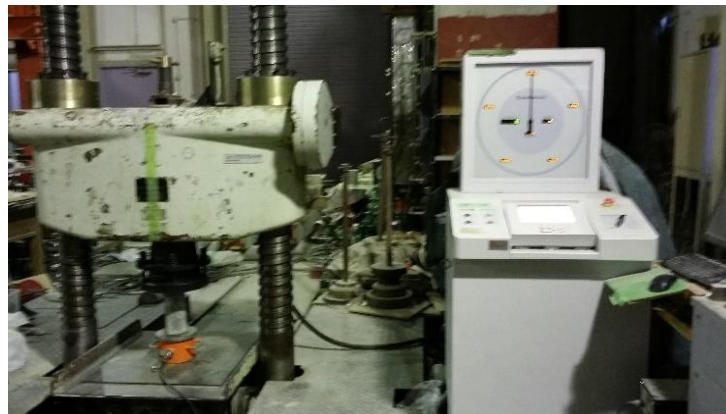
Figure 4. Test method for compressive strength of concretes .
