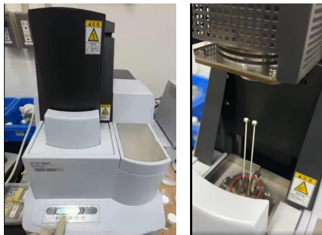
Figure 3. TG-DTA method for determining the \text{Ca}(\text{OH})_2 content in concrete.
